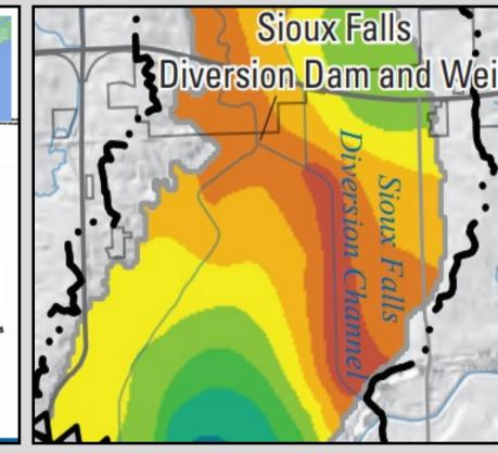
1961 diversion channel for flood Diversion Dam and Weil | control, Sioux Falls, South Dakota turned out to be a good recharge basin to replenish the local aquifer. Regular dredging of channel plus dam and weir operations combine to enhance recharge under normal conditions. Red zone in map on right shows high recharge zone (USGS 2019).
